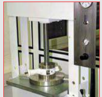
Thightness Test with Ultrapure Air
