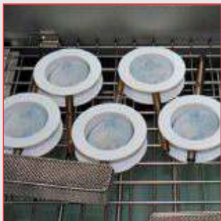
Cleansing the Parts with Ultrapure Water
